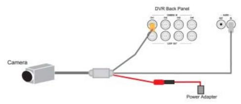
**Connection Type 2** – For cameras that have video/audio terminals on the rear panel of the camera body.
